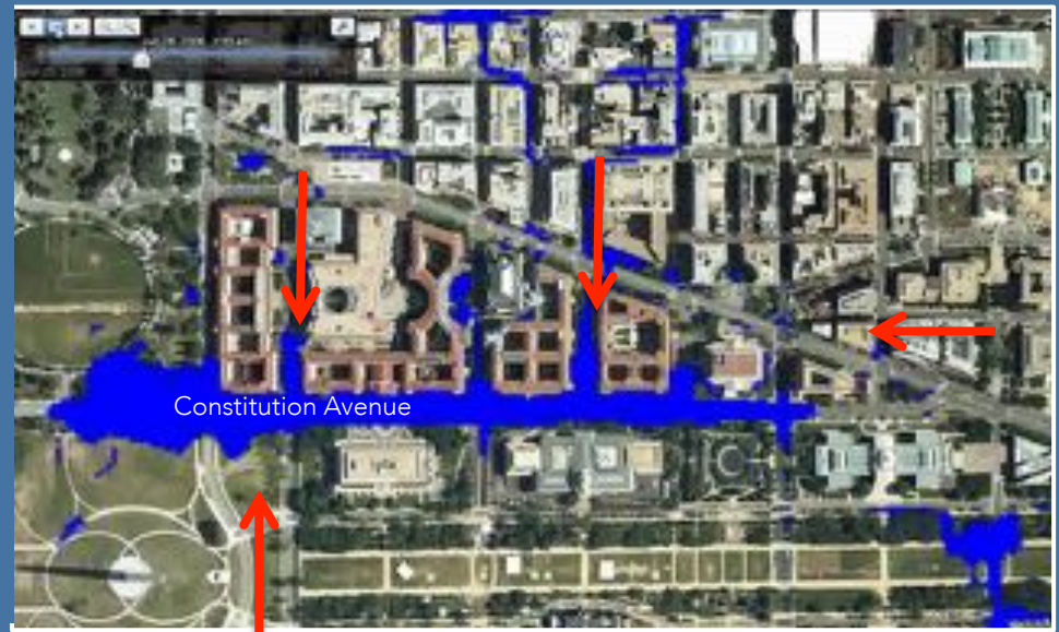
Blue areas show pooling of stormwater during the 2006 flood from runoff from higher ground (red arrows)
