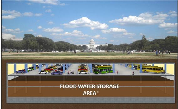
\*Sectional view represents an early stage concept from 2014. The revised 2017 concept reviewed by USACE has two stories: the upper story for cars would not be flooded; the lower bus level would be used for stormwater storage.
